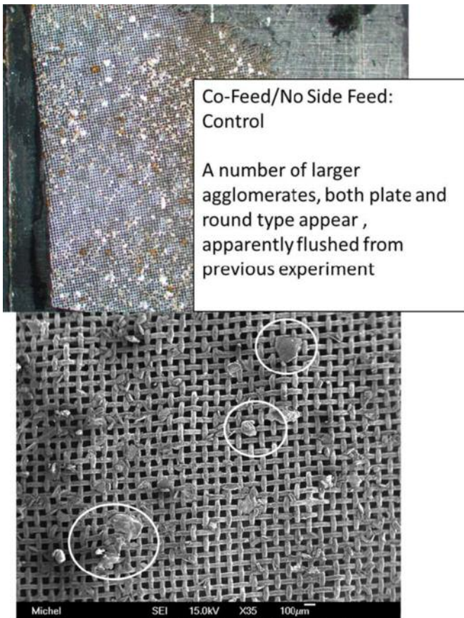
FIGURE 15 Screenpack screen after rear feed control for starve feed conditions after variable feeder flood feed conditions.
