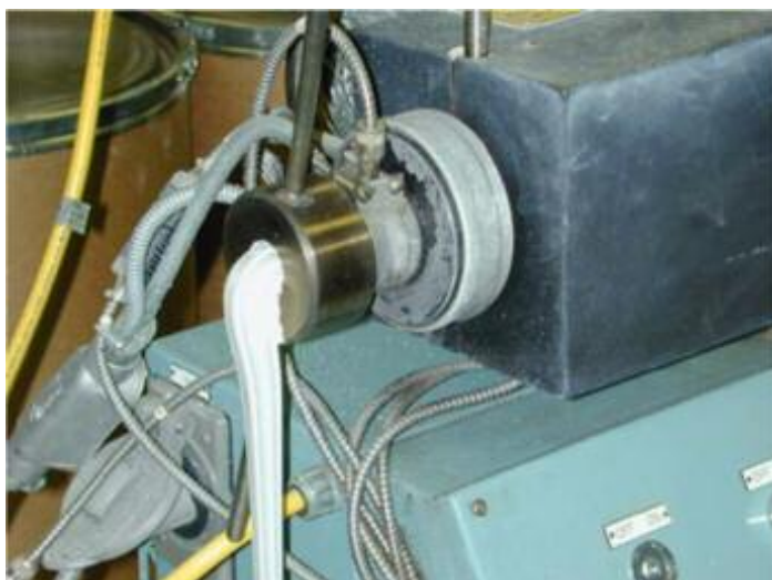
FIGURE 2 Purging TiO 2 masterbatch from debris fouled screenpack.
