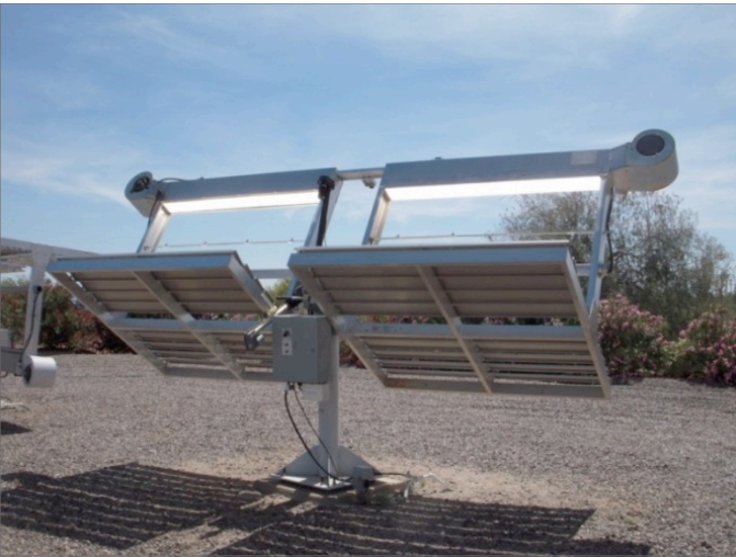
Figure 2. Fresnel-reflecting solar concentrator accelerated weathering apparatus
