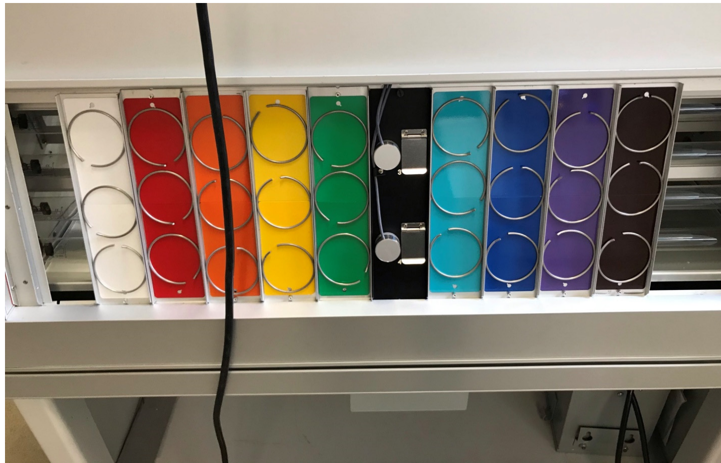
Figure 1. Painted metal panels mounted in a QUV/uvc tester
