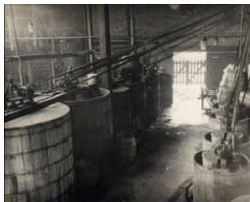
Fig. 7 Dye Coupling Tanks of Pharma Chemical ca. 1930. The Autoclave in Upper Left Was Part of the Original Distillery in 1914.
