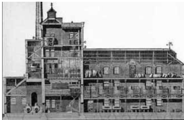
Fig. 1 Typical Multi-Story Brewery Designed for Gravity Flow
