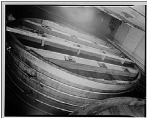
Fig. 3 Wood Lager Tanks Were Modified for Dye Manufacture.
