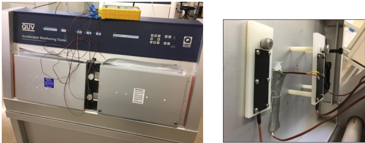
Figure 6. Fluorescent UV weathering chamber with three-dimensional specimen boxes on the front quadrants (left image). Test configuration for the front left 3D specimen box quadrant, view perspective from inside test chamber (right image) shows, from left to right: insulated black panel mounted to specimen box, chamber air, IBP on standoffs, BP on standoffs.
