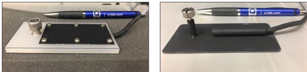
Figure 4. Black panel temperature sensor for xenon arc tester showing insulated (left) and uninsulated (right) configurations. Pen is included for scale.
