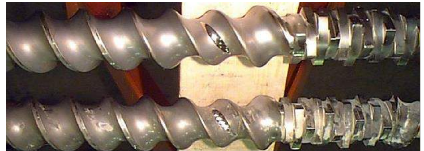
Figure 5: Wear due to back up into screw bushings. Flow direction left to right.
