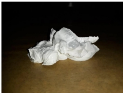
Figure 1. TiO 2 in mineral oil, no surfactants. A “solid” liquid.
